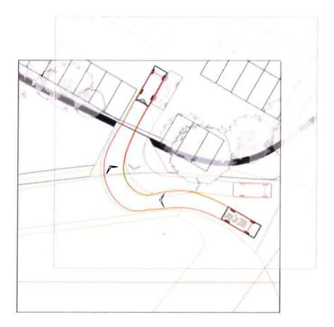
So the drawings do show that, the visibility splays can not be achieved with the current landscaping proposal, the cars turning out of the car park will not be able to see traffic turning in left from the Fosse until they are less than the stopping distance at 20mph appart and it is not possible to have a car turning in and a car turning out of the car park at the same time without them hitting each other. But this then all has a knock on (no pun intended) consequence....
